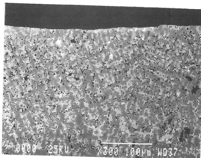
Figures 4 and 6 Scanning electron micrograph details of the polished section (see fig 3 for positions). Unetched. B.S.E. image. Both at same scale: white bar = 100 microns.
