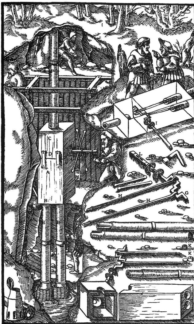
A—BOX. B—LOWER PART OF BOX. C—UPPER PART OF SAME. D—CLAMPS. E—PIPES BELOW THE BOX. F—COLUMN PIPE FIXED ABOVE THE BOX. G—IRON AXLE. H—PISTON-RODS. I—WASHERS TO PROTECT THE BEARINGS. K—LEATHERS. L—EYES IN THE AXLE. M—RODS WHOSE ENDS ARE WEIGHTED WITH LUMPS OF LEAD. N—CRANK.
