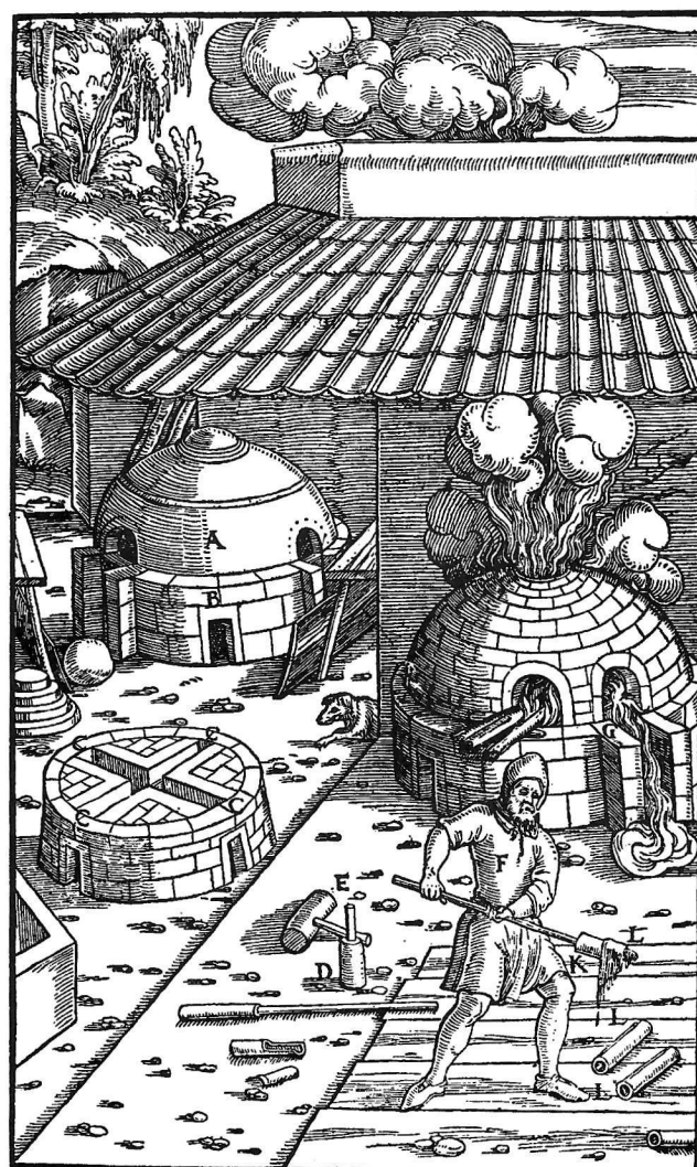
A—CHAMBER OF THE FURNACE. B—ITS BED. C—PASSAGES. D—RAMMER. E—MALLET. F—ARTIFICER MAKING TUBES FROM LITHARGE ACCORDING TO THE ROMAN METHOD. G—CHANNEL. H—LITHARGE. I—LOWER CRUCIBLE OR HEARTH. K—STICK. L—TUBES.
