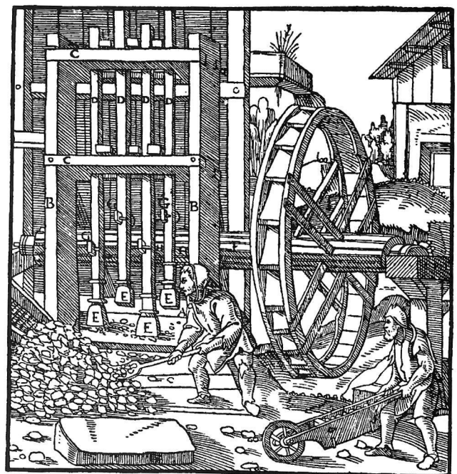
A—MORTAR. B—UPRIGHT POSTS. C—CROSS-BEAMS. D—STAMPS. E—THEIR HEADS. F—AXLE (CAM-SHAFT). G—TOOTH OF THE STAMP (TAPPET). H—TEETH OF AXLE.
