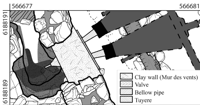
Figure 4: Plan of part of the blowery and the open hearth with the position of the devices embedded in the mur des vents added. Image width 4m.
