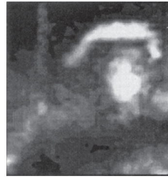
Figure 10: Raw earth resistance data over a 20m by 20m area at Timberholme showing a square structure. Clipped range 67 ohms (white) to 135 ohms (black)
