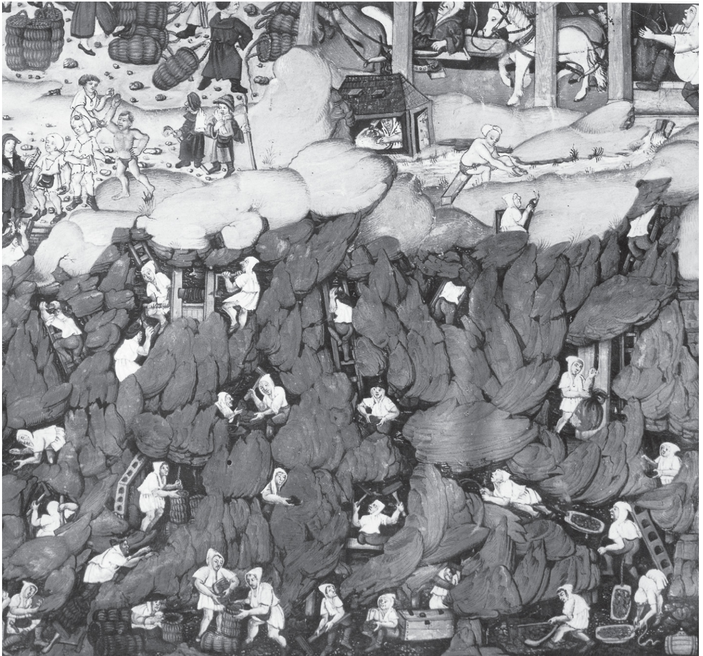
Figure 7a: Detail of the Kuttener Kanzionale , dated to the late 15th century (Haas and Kurzel-Runtscheiner 1929, Fritsch 1967), depicting medieval miners at work. Note the closed chests at the bottom which hold the silver-rich ore, while the low-grade ore is hauled in open trays (right). Photo Deutsches Bergbau-Museum, Bochum.
