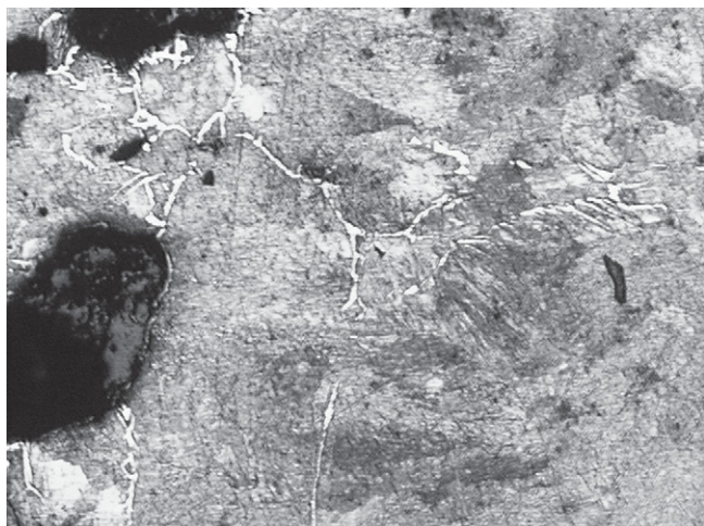
Figure 4: Sou 31/2780. Fine pearlite and bainite with grain boundary cementite indicating 0.8-1.2% carbon. Width of field 1280 \mu m.
