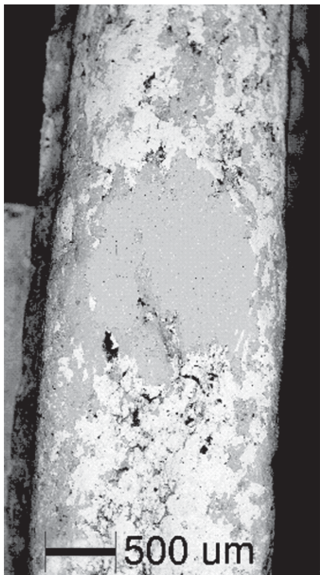
Figure 2: Edge of coin No. 7, showing tangential polished area (centre) and plating (pale areas above and below). SEM backscattered electron image.
