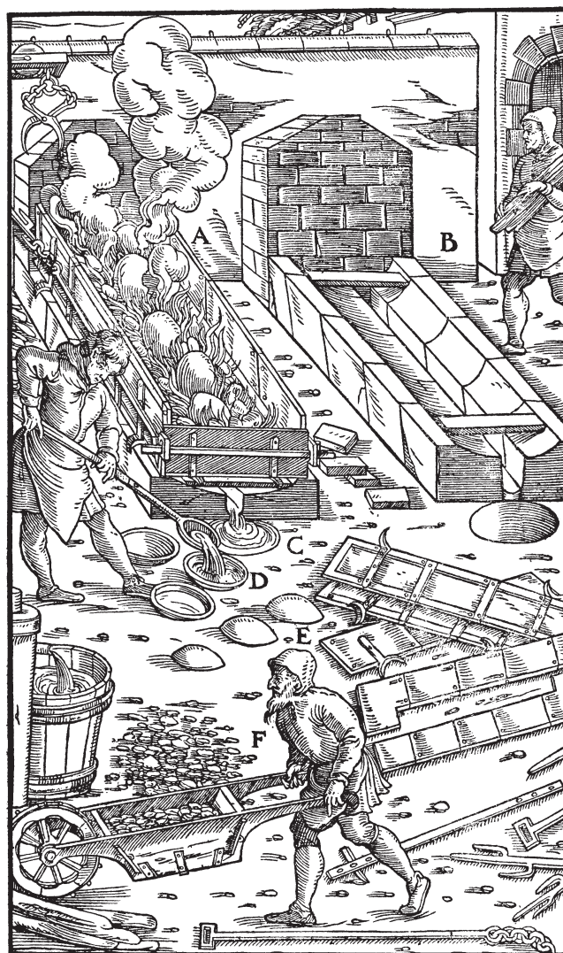
A—FURNACE IN WHICH THE OPERATION OF LIQUATION IS BEING PERFORMED. B—FURNACE IN WHICH IT IS NOT BEING PERFORMED. C—RECEIVING-PIT. D—MOULDS. E—CAKES. F—LIQUATION THORNS.
