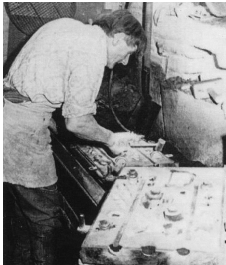
Figure 8: Photograph of the moulding operation in a Birmingham brass foundry. In the foreground a half-mould shows the pouring basin at the front, runner bar and mould cavities for several castings, some with cores already in position. Behind, the moulder is working on the other half-mould, tapping on the half-embedded patterns to loosen them before stripping from the sand. Photograph by, and by courtesy of, C McCombe
