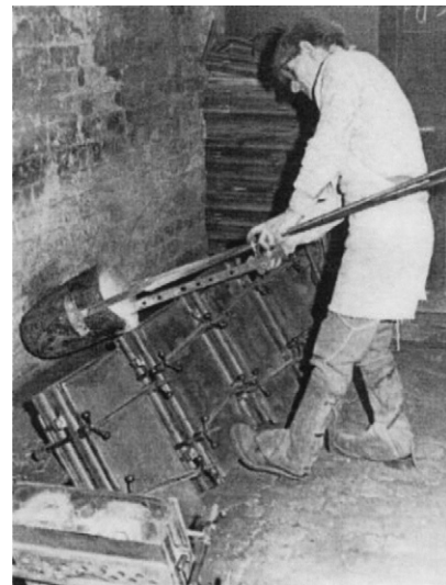
Figure 9: Photograph taken in the same foundry as Figure 8, showing the pouring of metal into the mould. The moulds are closed and clamped together and are standing on their ends to receive the molten brass, in this case from a crucible. At Bullows' the iron was melted in a larger cupola furnace and would have been poured from a ladle with a handle at the side. Photograph by, and by courtesy of, C McCombe
