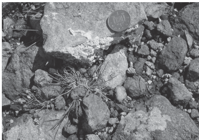
Figure 2: Type 1 light-coloured slag coating on a piece of sandstone (below and left of coin), from Calver 72A.
