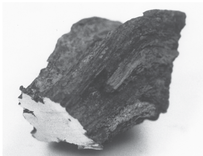
Figure 4: Piece of wrought-iron hoop showing the cut surface (Fig 3, area C).
