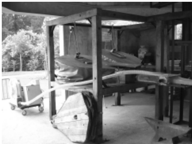
Figure 7: The ventilation system. For now the electric blower replaces the bellows.
