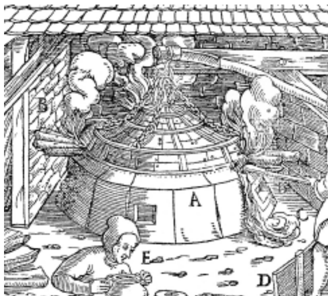
Figure 1: One of the furnaces for large-scale cupellation illustrated in De re metallica .
