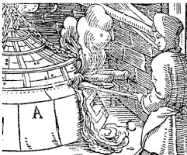
Figure 13: Drawing out of the litharge (C) illustrated in De re metallica .
