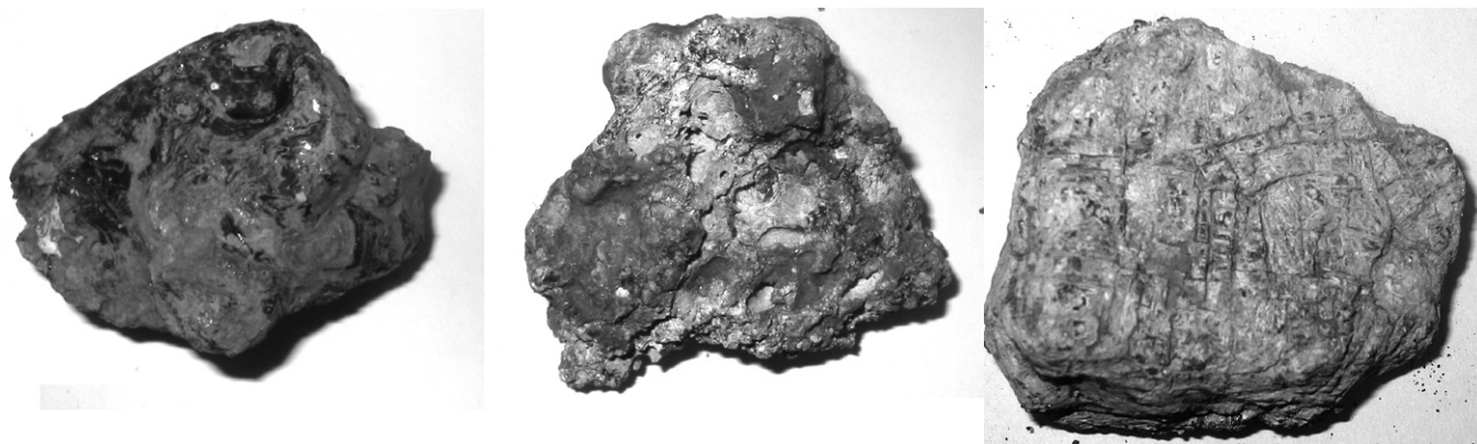
Left to right, Figure 4: Slag sample from trench 5, width 60mm. Figure 5: Furnace wall associated with slag from trench 6, width 66mm. Figure 6: Galena sample from trench 6, width 46mm.
