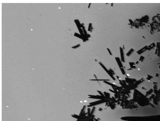
Figure 11: Secondary electron image of sample 5-4c showing the glassy matrix (light grey) and associated alumina-silicates (dark grey) and sulphides (white). Image width 200µm.
