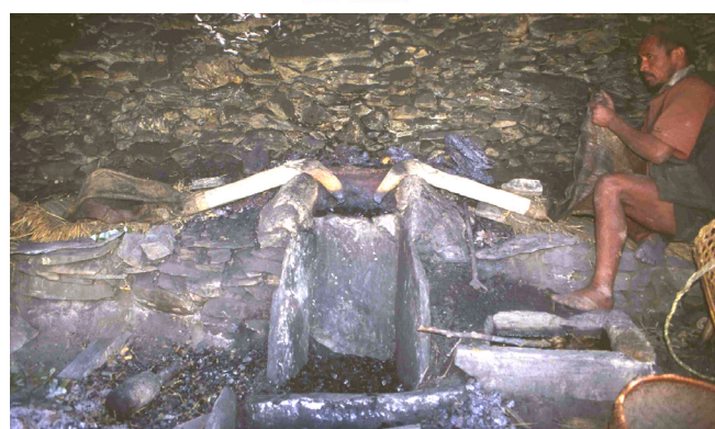
Figure 8: a) Copper matte smelting process of chalcopyrite ores by Nepalese smiths in Sikkim as recorded in the 1850s by Blandford and reported in Percy's Metallurgy . B) The process that continued at the village of Okharbot in western Nepal until the 21st century.
