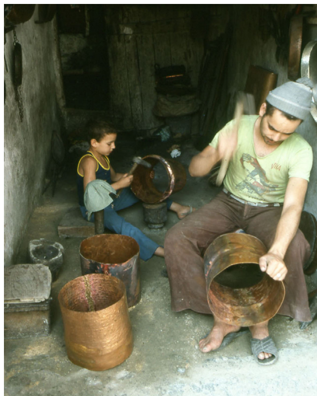
Figure 7: Traditional copper smith at Fez, Morocco in 1985, but the vessel was made from sheet copper bought in from a stockist, not raised or sunk in a traditional manner.
